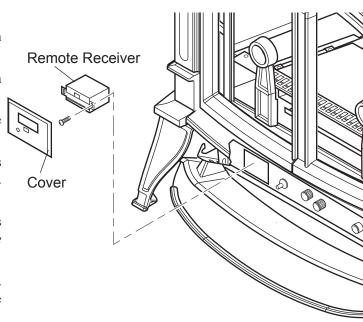
Figure 11 - Installing Remote Receiver
